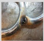
Tack to lightly secure the pieces. Evaluate the orientation. Adjust if needed by breaking the tack.
