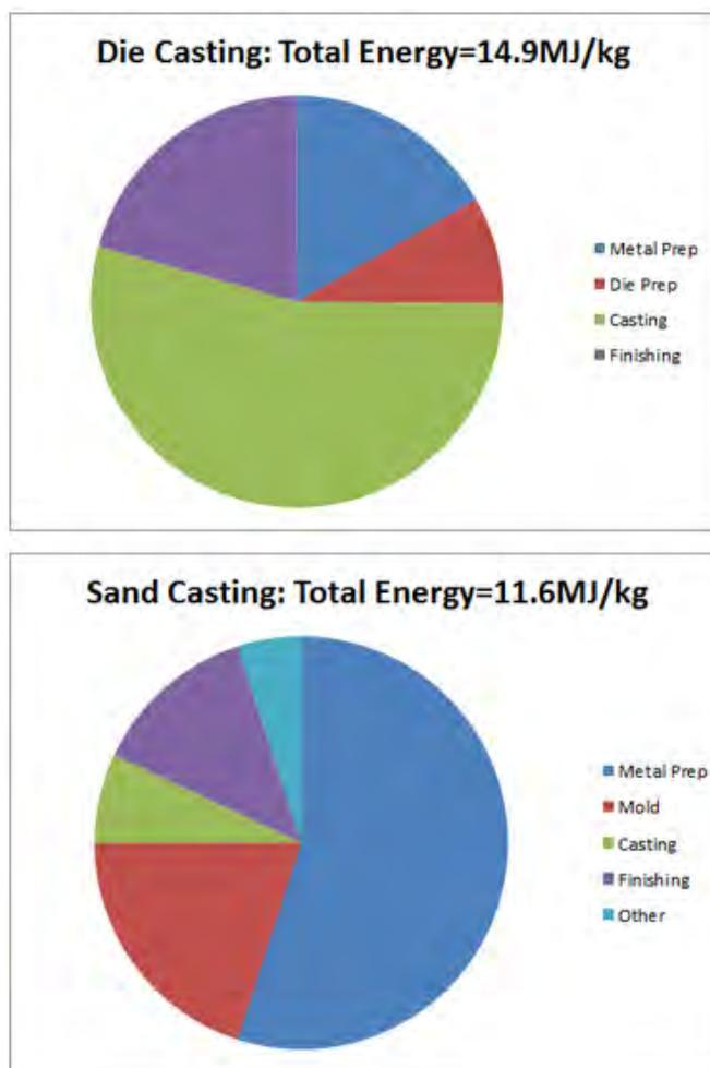
Fig. 16. A comparison of the environmental impact of sand and die casting
