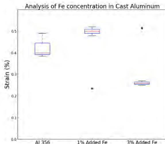
Fig. 7. Box and whisker plot of the maximal elongations of the lost wax cast dog bones. The outliers noted in red and are likely due to casting defects.
