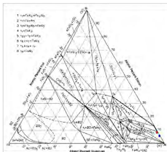
Fig. 11. Al-Si-Fe phase diagram at 600°C. Alloy A356 is represented by the blue dot, and A03320 is represented by the red. Modified from [4].
