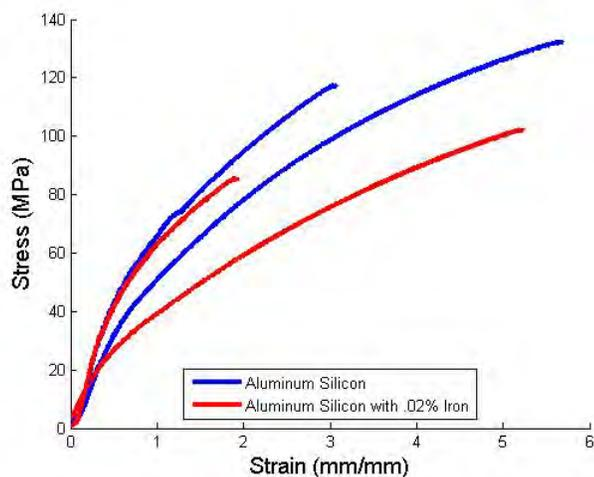
Fig. 4. Stress strain curves for the sand cast dog bones
