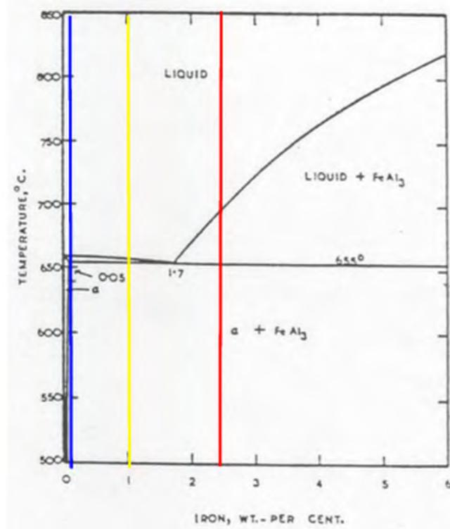
Fig. 6. The relevant part of the Al-Fe phase diagram, with some important regions highlighted. [9]
