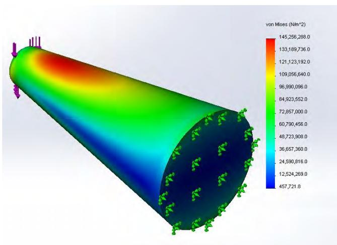
Fig. 15. This is a possible redesign of the leg of the pot. The maximum stress experienced here is 145 MPa, and since this is closer to the yield strength of aluminum, 192 MPa [12], a drop in this orientation probably would not cause fracture. If the pot was malleable or ductile cast iron, with a yield strength in the range of 224 MPa-864 MPa [14], it would not have experienced failure.
