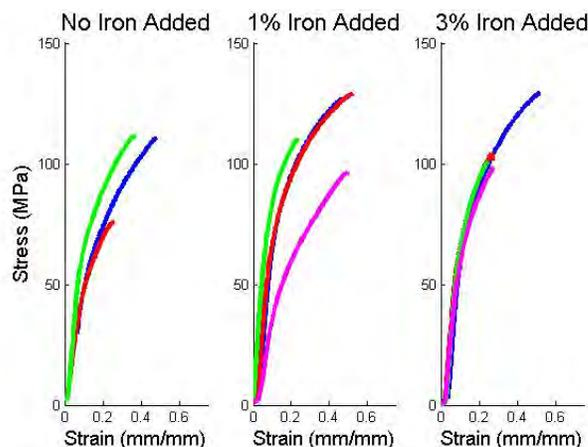
Fig. 8. Stress strain curves for the wax cast dog bones of A356, A356 with 1% added iron and A356 with 3% added iron
