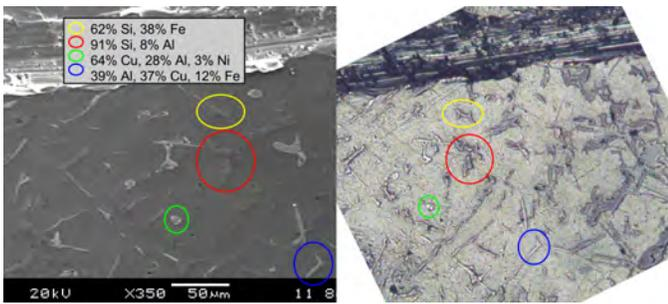
Fig. 2. The zambian pot under the SEM (left) and optical (right) microscopes. Circled areas highlight specific elements of the microstructure.
