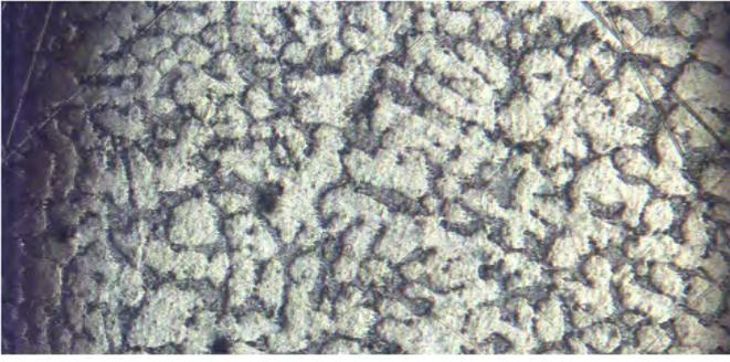
Fig. 12. The commercial Al-Si alloy at 200x magnification.
