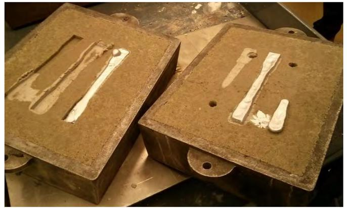
Fig. 3. The mold and sand cast dog bones
