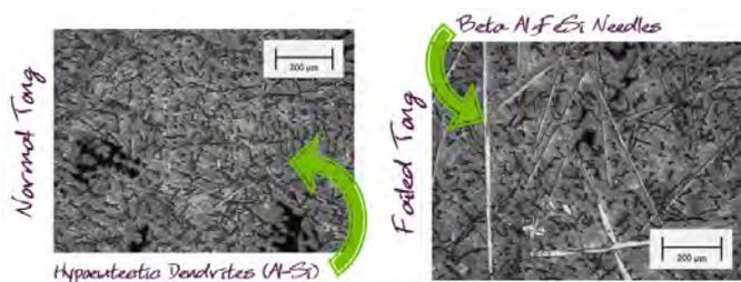
Fig. 5. Comparison of the normal and failed tongs from [8]. The iron content of the failed tong was much higher than that of the normal tong.
