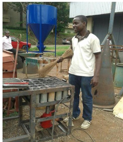
plate 3.12: Pistons at top dead center after briquette ejection
