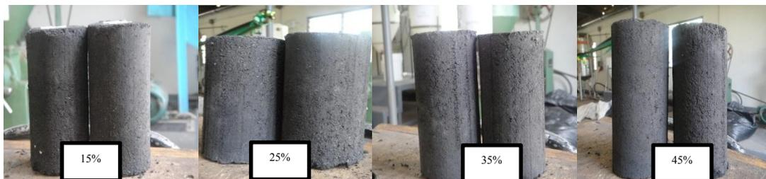
Plate 3.8: Briquette of particle size less than or equal to 2mm at different binder level after drying
