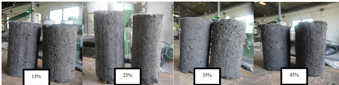
Plate 3.7: Briquette of particle size less than or equal to 6mm at different binder level after drying
