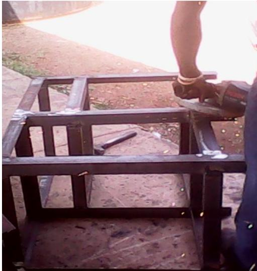
Plate 3.4: Frame under construction
