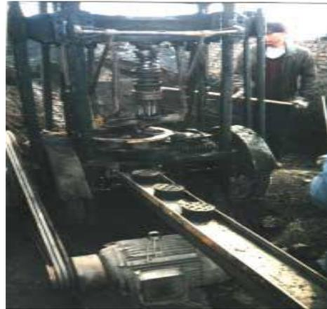
Plate 2.2: Chinese semi-mechanised briquetting press (Beijing, 0086/10/677 812 07)
