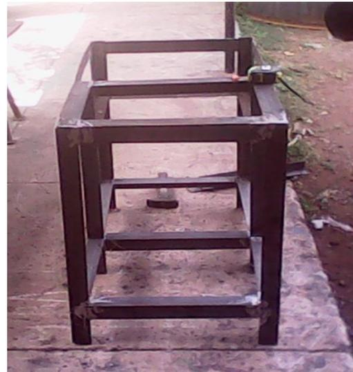
Plate 3.5: Frame after construction
