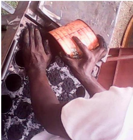
Plate 3.9: Biomass loading stage
