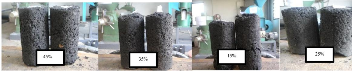
Plate 3.6: Briquette of raw char (original particle size) at different binder level after drying
