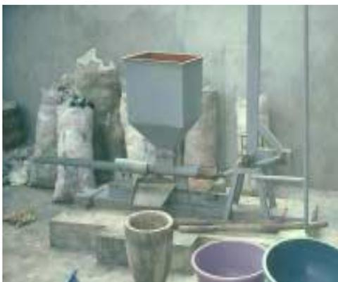
Plate 2.3: Manual briquetting press for biomass and waste paper in Benin (DCAM, 00229/321129)
