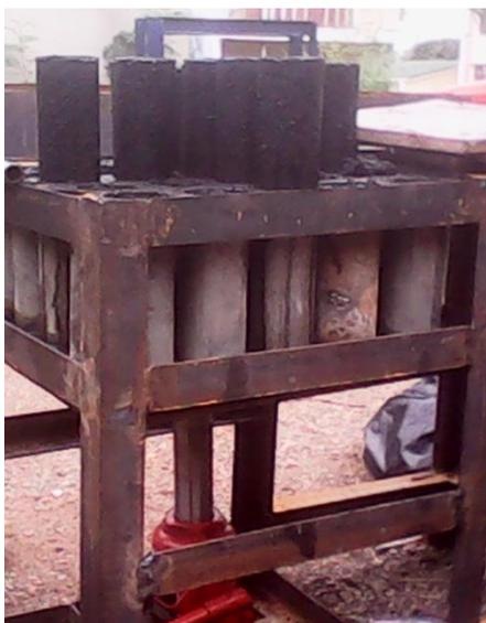
Plate 3.11: Briquette ejection stage
