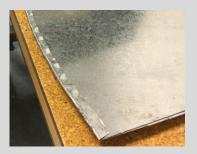
15. Fold the bottom edge along the sketch drawn earlier until the tab is at a 90° angle. This bend should be made such that the tab faces outward from the bucket.
