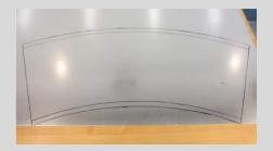
Use the correct directional snips. For the straight edges, use the straight snips. For the top and bottom arcs, use the correct directional snips that orient in the way that the arc curves.
