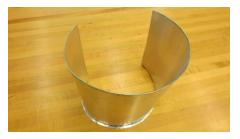
Teaching note: Demonstrate that should the bottom tab kink, the participant should rotate the sheet metal to flatten out the kink against the table surface. This will effectively thin the sheet metal in that area.
