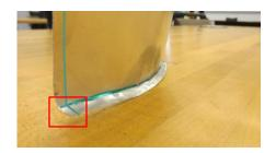
18. Fold each of the two straight edges almost completely over (more than 90 degrees), with an offset of about ½" (1.3cm). These two edges are meant to hook together, and are therefore folded in the same direction.
