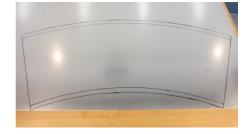
13. Use the curved snips to cut along the top and bottom arcs of the bucket pattern and straight snips for the sides.
