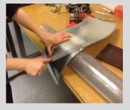
Keep shaping the sheet metal until you feel as though the two edges can touch with little force applied. Only until you are confident of this step can you move on.
