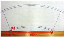
6. Place the drawing tool on the table or floor such that the marker will touch both marks when the string is taut.
