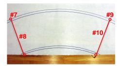
12. Cut out the butcher paper sketch and determine whether it will create a bucket as desired. After adjustments are made, transfer the sketch to the sheet metal.
