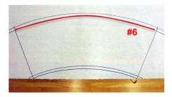
11. Remove the marker from the string. Stretch the string so that it intersects one of the two end points of the smallest arc. At that position, mark where the string intersects the largest arc. Repeat for the other side. Connect the marks on the largest and smallest arcs with a straight edge to form the sides of the bucket.
