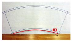
8. Release the string knot slightly so that the length of the string is just over 25" (63.5cm). Draw another arc. This will give a guideline for bending the bottom edge of the bucket.
