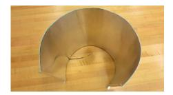
19. Hook the two folds together and use the flat bar to fully flatten the seal. If needed, insert the round object into the bucket to create a surface against which to shape the sheet metal.
