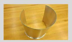
17. To connect the sides of the bucket, a small piece of sheet metal needs to be removed. From one of the ends, cut off a portion of the tab that is equal to the width of the intended fold for the seam.
