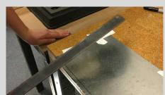
Use the table's edge. Make changes gradually. The approximately ¼" to ½" (0.64cm to 1.3cm) of sheet metal below the drawn line should be over the edge of the table. Using a downward trajectory and relying on the edge of the table to facilitate the bend, begin shaping this tab. Changes should be made incrementally, from right to left, then back again, to ensure that the metal is shaped slowly and does not develop any kinks.
