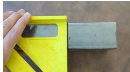
2. Mark the same line along all sides of the metal tubing. Also, mark a 1/2" (1.3cm) long line starting at the top of the tube and going down along every corner.
