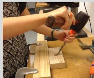
*Using both chisels.* As you remove more material with the smaller chisel, the hole will become deeper. As this happens, it is important to redefine the edges of the hole. Make vertical cuts with the large chisel as needed to mark the edges of the hole. Near the end of the hole, it is important to remove even smaller pieces of the wood as it is more likely to split the closer the bottom of the hole is to the bottom of the wood.
