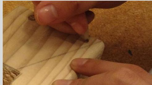
*Placing the nail.* Begin by nailing into the first piece, before placing the two pieces together and nailing into the second piece. To ensure the nail is in the correct position, hold it at an angle, resting the point on the drawn mark. Then, straighten the nail, creating a small indent on the mark.
