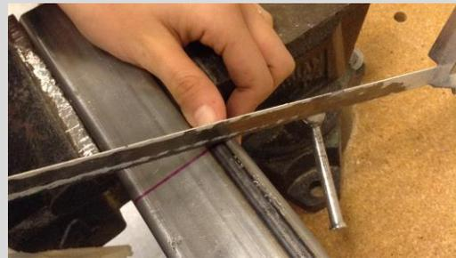
*Let the saw do the work.* Choosing a saw with the appropriate number of teeth per inch is important to using a hacksaw efficiently. More teeth per inch should be used on thinner material while fewer teeth per inch should be used on thicker material. For cutting pipe, more teeth per inch will make for a smoother cut and the blade will catch less.
