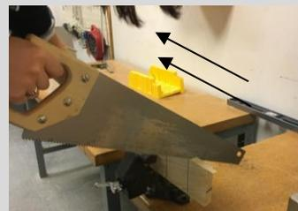
*Sawing.* Hold the saw at a 45 degree angle from the horizontal as you cut. Start moving the saw back and forth. Not much pressure is needed, it is better to let the saw do most of the work. As you get near the end of the cut, slow down the pace of the saw to avoid splitting the wood.
