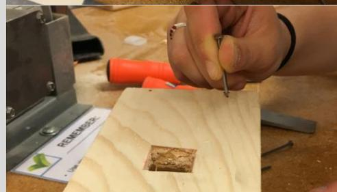
*Hammering.* Hold the nail firmly to keep it straight with driving it into the wood. It will tend to lean at an angle if not held in place, which leads to the wood potentially splitting or the sharp point of the nail poking out of the finished product. Start by holding the hammer close to the head for control. Once the nail is firmly in the board, hold the hammer further away from the head for power. Drive the nail in until its head is flush with the board's surface.
