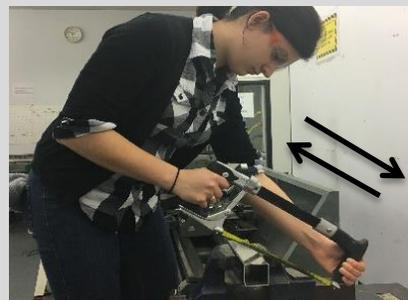
4. Use the hacksaw to cut downward along the  $\frac{1}{2}$ " (1.3cm) lines drawn at the corners to form the tabs.
