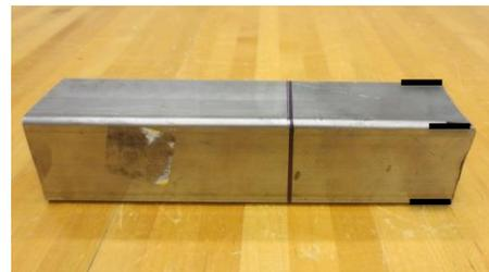
3. Place the metal in the vice. Use the hacksaw to cut along the line drawn such that a 3.5" (9cm) piece of metal tubing is produced.
