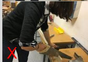
*Starting the cut.* Place the saw on the cut line. Pull the saw back along the top edge of the wood until a groove is formed. This will help guide the blade as you start sawing.
