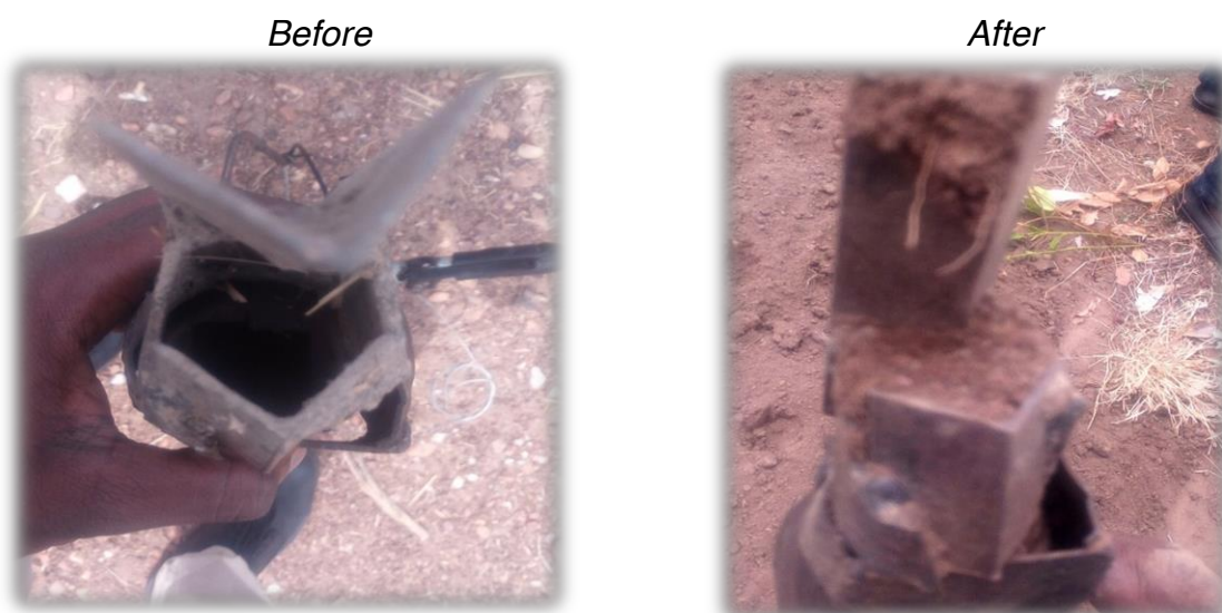
Fig. 8. The furrow cutter got plugged with moist soil.
