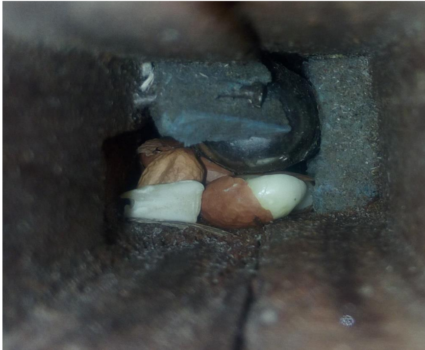
Figure 9. Peanuts stacked and bruised at the metering device
