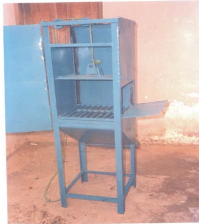
Fig. 2.3 Picture showing manually operated cocoa depodding machine designed by Adewumi & Fatusin.
