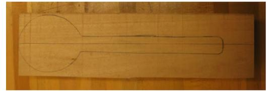
3. The rim of the spoon should be of an even thickness. Sketch a line for the inner edge of the rim and cut out the shape.
