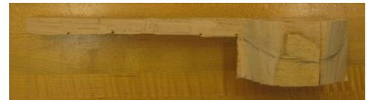
15. Using both the coping saw and chisel, where appropriate, remove the rest of the excess material around the bowl.
