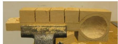
11. Turning the spoon on its side, sketch the side profile of the handle.
