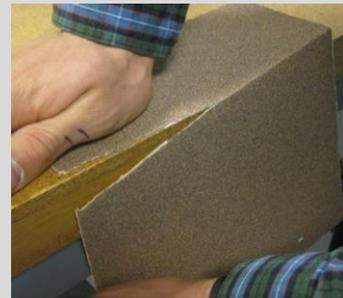
*Create sanding blocks.* One can use more force in sanding by creating sanding blocks as oppose to holding the sand paper in one's hand. The simplest sanding block can be made by stapling a piece of sand paper to a scrap of wood. When stapling the sand paper, ensure the two ends have folded over each other. This will prevent the sand paper from easily ripping off the block. Keep a portion of the block uncovered so one's hand isn't directly gripping the sand paper.
