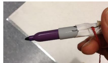
3. Tie the string to the nail such that the distance between the nail and the marker measures 35" (89cm) when taut. The length of the string affects the rate of curvature for the top edge of the bucket.
