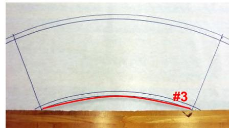
8. Release the string knot slightly so that the length of the string is just over 25" (63.5cm). Draw another arc. This will give a guideline for bending the bottom edge of the bucket.
