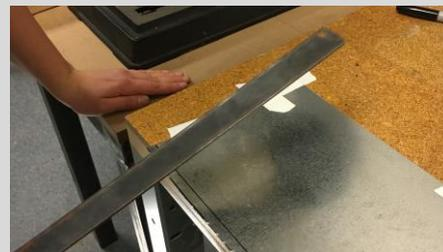
*Use the table's edge.* Make changes gradually. The approximately  $\frac{1}{4}$ " to  $\frac{1}{2}$ " (0.64cm to 1.3cm) of sheet metal below the drawn line should be over the edge of the table. Using a downward trajectory and relying on the edge of the table to facilitate the bend, begin shaping this tab. Changes should be made incrementally, from right to left, then back again, to ensure that the metal is shaped slowly and does not develop any kinks.
