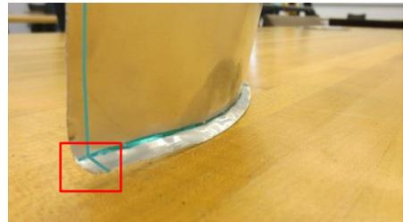
18. Fold each of the two straight edges almost completely over (more than 90 degrees), with an offset of about 1/2" (1.3cm). These two edges are meant to hook together, and are therefore folded in the same direction.
