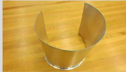
17. To connect the sides of the bucket, a small piece of sheet metal needs to be removed. From one of the ends, cut off a portion of the tab that is equal to the width of the intended fold for the seam.
