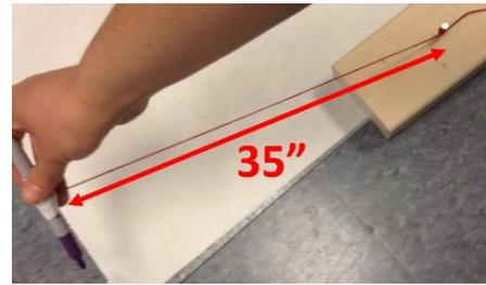
4. From the marker attached to the string, measure 25" (63.5cm) and mark this point on the string. Tie the string around the nail so that the 25" (63.5cm) length is free to draw a circle. The difference between this value and the previous value is the approximate height of the bucket. In this case, that is 10" (25cm).
