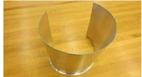
*Teaching note: Demonstrate that should the bottom tab kink, the participant should rotate the sheet metal to flatten out the kink against the table surface. This will effectively thin the sheet metal in that area.*
