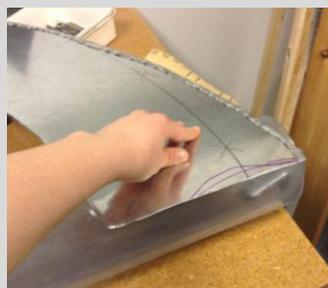
*Begin shaping the sheet metal against the round object with the flat bar. Work from the right-most edge to the left-most edge of the sheet metal. Do this incrementally so that the metal does not have any kinks. Further, take pauses to shape the bottom tab so that it remains flat and at 90 degrees.*
