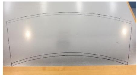
13. Use the curved snips to cut along the top and bottom arcs of the bucket pattern and straight snips for the sides.
