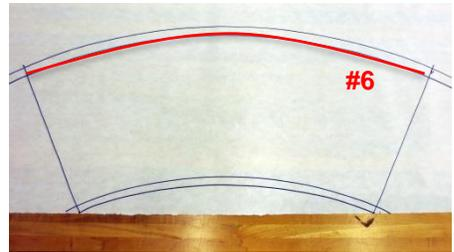
11. Remove the marker from the string. Stretch the string so that it intersects one of the two end points of the smallest arc. At that position, mark where the string intersects the largest arc. Repeat for the other side. Connect the marks on the largest and smallest arcs with a straight edge to form the sides of the bucket.
