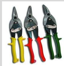
*Place the metal into the mouth of the snips.* Make sure that the sheet metal is inserted as far as possible into the mouth when cutting.
