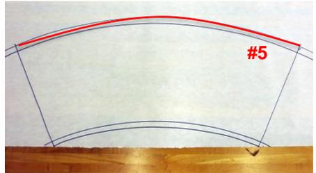
10. Double knot the string and draw a final arc. This one will be slightly inset from the previous line, and provides a guideline for bending over the top edge.
