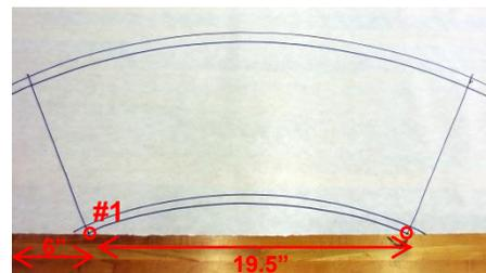
6. Place the drawing tool on the table or floor such that the marker will touch both marks when the string is taut.
