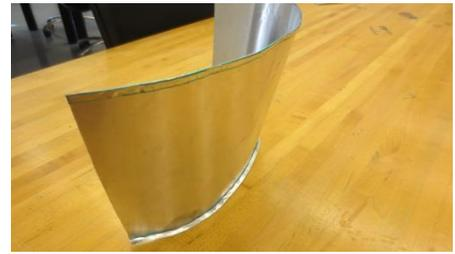
16. Shape the sheet metal into a circle so that the straight edges will touch when very little force is applied. Use a round object as a surface against which to shape the metal.
