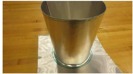
21. Fold the edges of the circle in along the inner outline. Once the edges are folded 90 degrees, place the bucket inside the circle aligned with the outline made previously and continue to fold the edges over until they are flat. Now, the tab on the bottom edge of the bucket is sandwiched in the fold.
