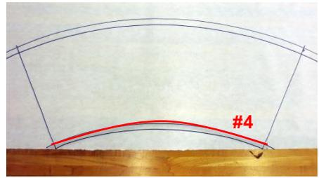
9. Fully untie the knot in the string made earlier so that the drawing radius measures 35" (89cm). Keeping the block in the same location, draw another arc as long as is allowed by the amount of butcher paper.
