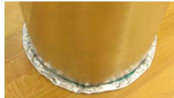
22. Finally, fold the entire edge up so that it is flush with the sides of the body. This will ensure that the bucket is as water-tight as possible.
