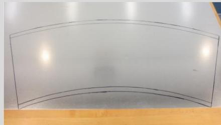
*Use the correct directional snips.* For the straight edges, use the straight snips. For the top and bottom arcs, use the correct directional snips that orient in the way that the arc curves.
