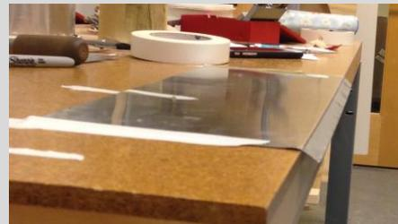
*Change angle and leverage as needed.* Once the tab has been folded 90 degrees, flip the sheet metal over so that the tab faces upward. Begin shaping the fold with the flat bar using the top of the table as the counter surface. Again, work from right to left and back again. Keep working until the tab is completely flattened against the sheet metal and there are no gaps between it and the rest of the sheet metal.
